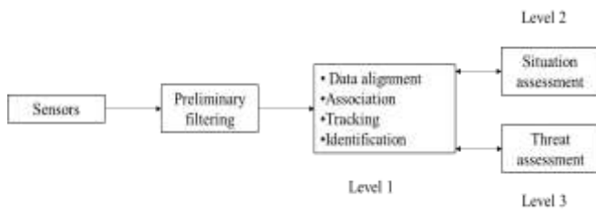
Fig. 5. JDL data fusion Architecture
